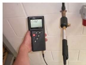
Pressure-tight moisture probe for measuring in compressed air
