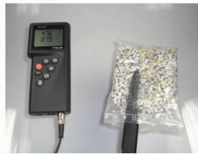
Measures equilibrium moisture in masonry, cement, plastic granulate
