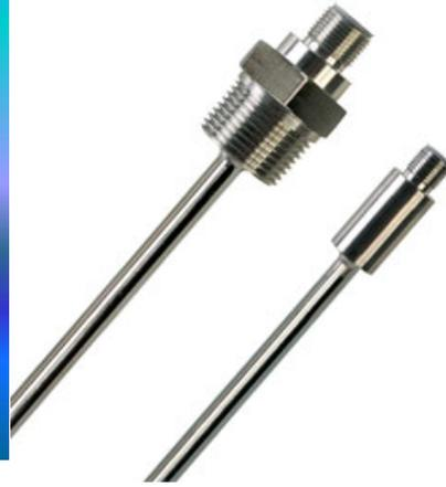
RTD sensors are made with 316L Stainless Steel housings for strength and corrosion resistance. These sensors include a 4-pin, M12 plug connector for easy assembly to patch cables or extension cables, as well as NPT, BSP pipe threads and two metric mounting thread options for easy installation into an existing threaded port. A non-threaded housing option is also available for other types of installations.
