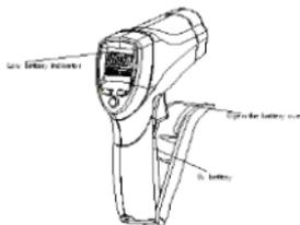
② Open battery cover, then take out the battery from instrument and replace with a new 9-Volt battery and place the battery cover back.
