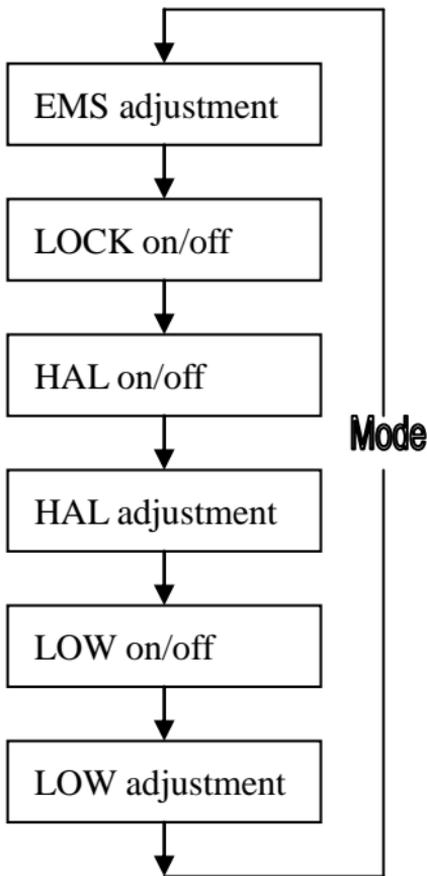
Press the mode button also allows you to access the set state, Emissivity(EMS), Lock on/off, HAL on/off, HAL adjustment LOW on/off, LOW adjustment, Each time you press set you advance through the mode cycle. The diagram shows the sequence of functions in the mode cycle.
