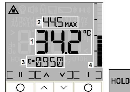
After taking a measurement the following functions can be displayed in turn by pressing the **▲**-button (starting from the **HOLD** mode):
