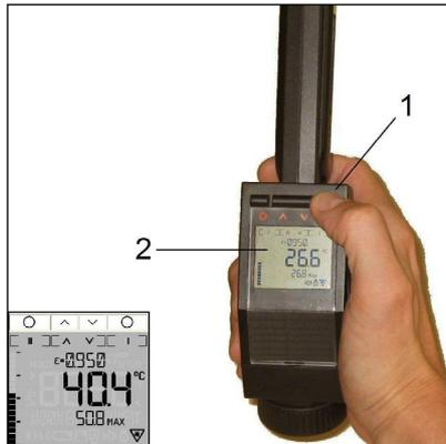
**On**, the **I**-button automatically gets the function of the **Trigger** [1] and the readings in the display [2] are turned by 180° **[► Flip-Display]**.
