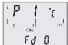
Push [ENTER/MENUE] to confirm. On the display appears **00.00**. For changing the value use the up key [▲]. For stepping to the next number use the down key [▼]. If the requested value is complete then push [ENTER/MENUE] to confirm.
