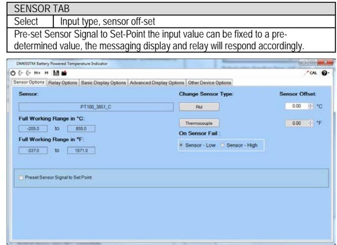
DM650TM configuration software (Sensor Options Tab).
